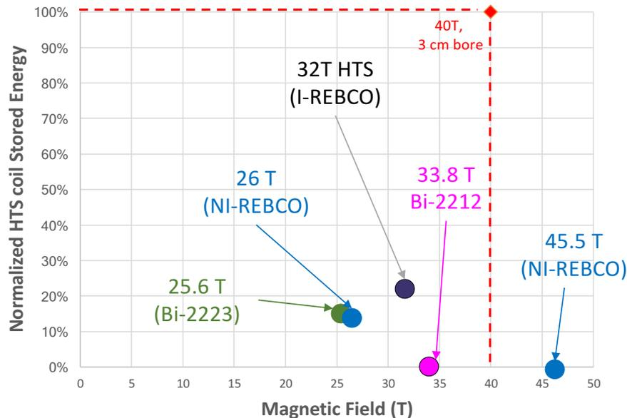
The MagLab is starting to develop a 40 T, 3 cm bore magnet for CMP. (Similar in size to 30 T, 10 cm bore.)
