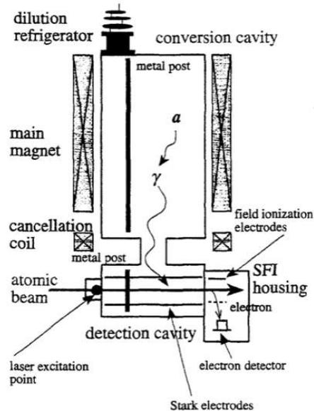
Figure 1. Schematic diagram of CARRACK II experimental system.
