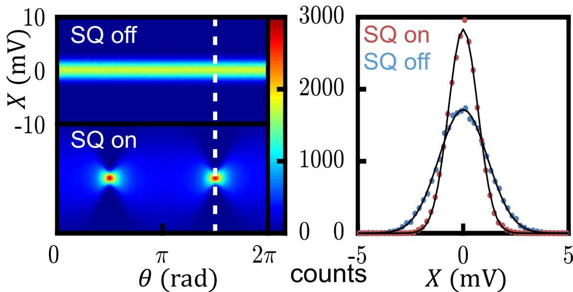
$$\frac{\sigma_{\text{off}}^2}{\sigma_{\text{on}}^2} = 4 \text{ dB}$$
