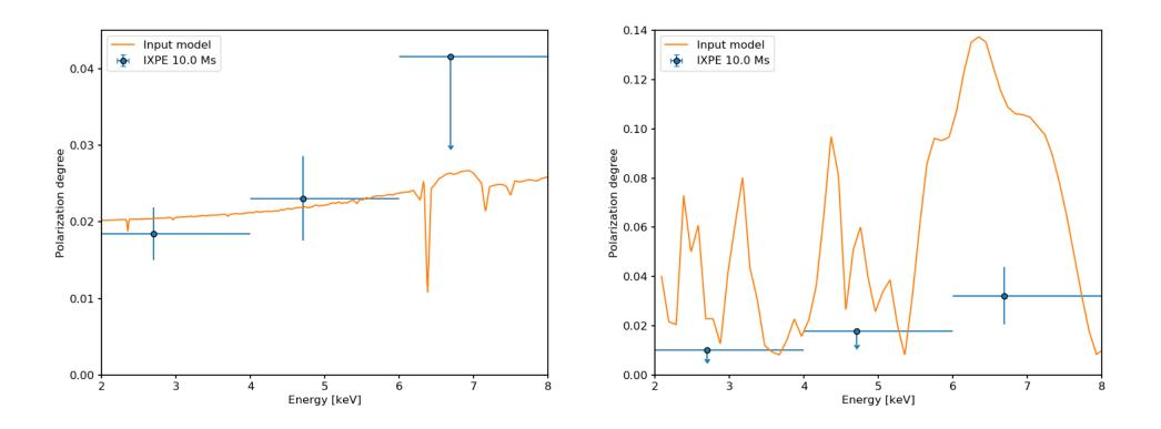
The linear polarization angle of a type-2 AGN in the absence (left) and presence (right) of axions.
