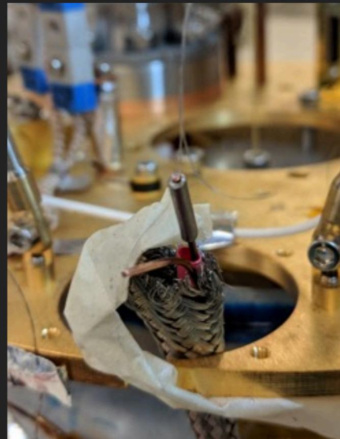
Superconducting solder capillary shield!
