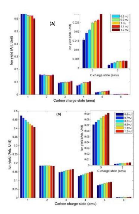
Carbon Ion Fragment Charge State Distribution Dependence on the FEL Pulse Energy
