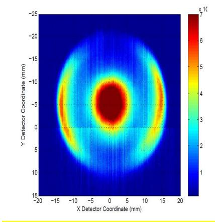
Electron spectra recorded for ionization of Ne. Outer ring: Ne 1s photoelectron diplole angular distribution.
