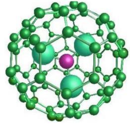
Use pump-probe technique, 10 fs pulses of 1400– 1500 eV photon energy, to track the evolution of ionization and fragmentation of Ho<sub>3</sub>N@C<sub>80</sub>.
