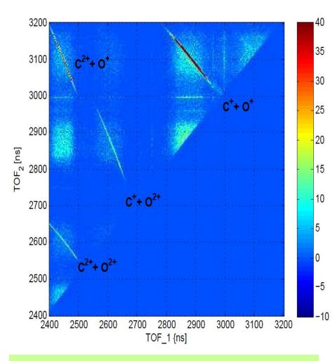
Ion-Ion Coincidence Events recorded during ionization of CO with 430 eV X-rays with 5fs pulse duration.
