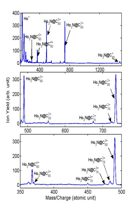
Multiphoton X-Ray Induced Fragmentation of Ho<sub>3</sub>N@C<sub>80</sub> at LCLS
