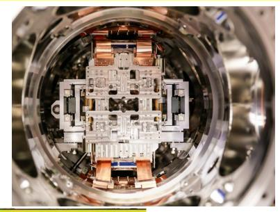
MPI Semiconductor Lab (Munich): 1024x1024 pixels pixel size: 75 x 75  $\mu$ m<sup>2</sup> active area: 59 cm<sup>2</sup> frame rate: up to 200 Hz single-photon resolution up to 10<sup>3</sup> photons (1keV) per pixel  $\Delta$ E/E~5% (800eV to 2000eV) Q.E.  $\geq$  90 % from 0.8 to 10 keV operating range 0.1 < E < 25 keV
