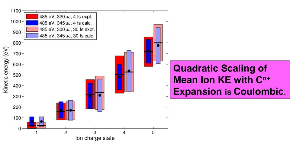
Mean ion kinetic energy: circles (experiment) and lines (simulation). RMS kinetic energy width: Height of each rectangle.
