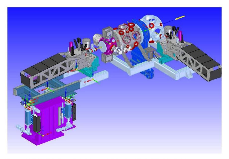
Figure 1: CAD model of the spectrometer installed on the AMO LAMP instrument. Two configurations, forward and 90° horizontal are shown.
