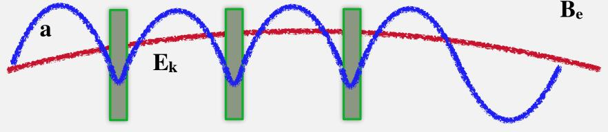
• Dielectric layers distort the free photon wave function, giving a non-zero overlap
