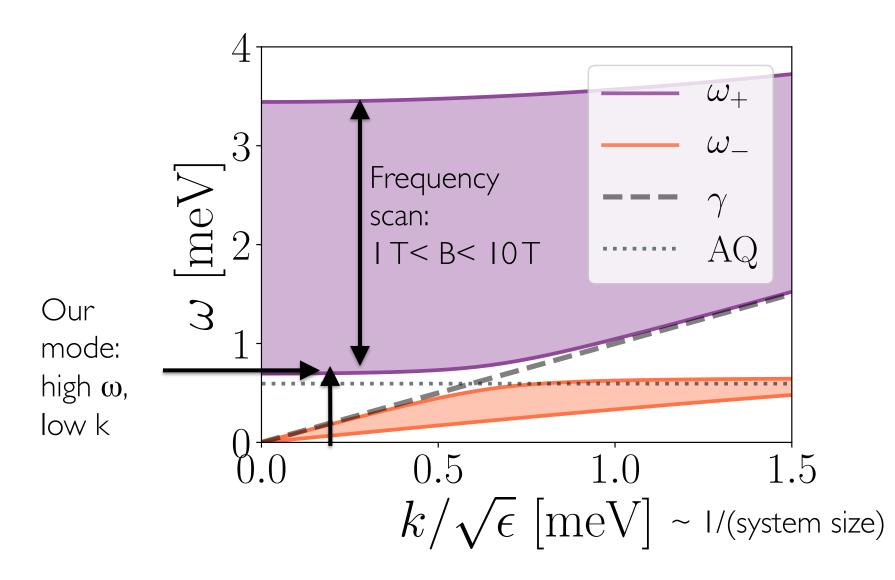
$\phi_+$  polariton has non-zero frequency at k=0, i.e. massive scalar particle.  $\rightarrow$  Long wavelength, large volume THz mode for detection. Basic concept: AF-doped TIs  $\rightarrow$ tunable THz resonance coupled to the axion.V = V<sub>sample</sub>
