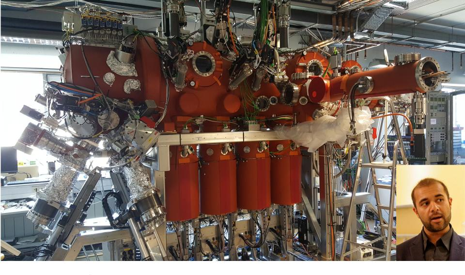
Making thin film heterostructures. "Mango": hybrid deposition tool. MPI Microstructure Physics, Halle.
