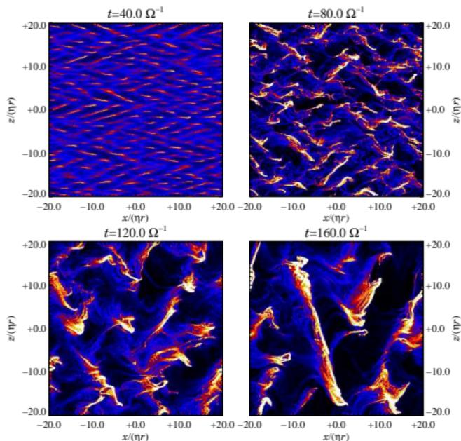
The radial drift flow of solids is linearly unstable!
