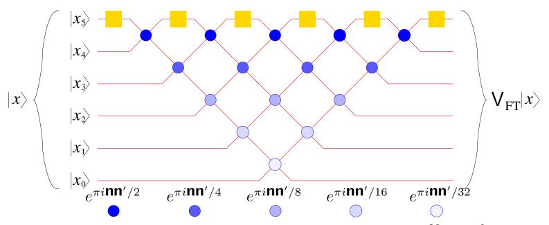
Since only top 20 layers of phase gates matter when  $N > 2^{20} = 10^6$ , time for QFT scales not quadratically but linearly in number of Qbits.
