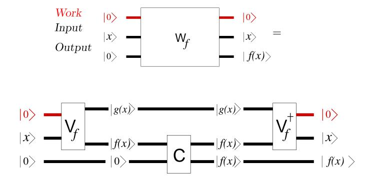
${\bf C}$  is built out of 1-Qbit controlled-NOT gates:
