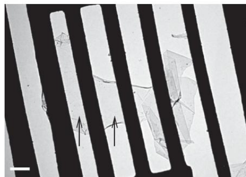
Figure 1 | Suspended graphene membrane. Bright-field TEM image of a suspended graphene membrane. Its central part (homogeneous and featureless region indicated by arrows) is monolayer graphene. Electron diffraction images from different areas of the flake show that it is a single crystal without domains. We note scrolled top and bottom edges and a strongly folded region on the right. Scale bar, 500 nm.
