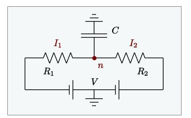
System: central capacitor, n: particle/charge number M=2 reservoirs, symmetric barriers
