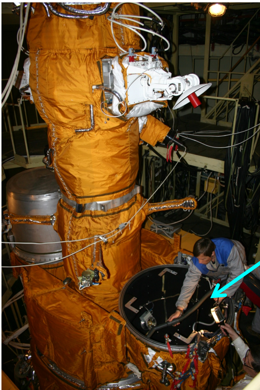
PAMELA INTEGRATION in the RESURS-DK1 satellite
