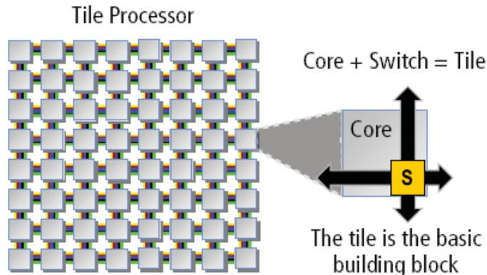
**64 cores connected in a mesh**
