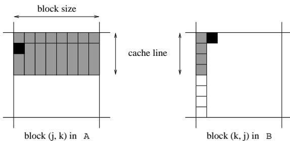
The block size must not be too large. Must be able to hold all the grey elements in **A** in cache (until they have been used).
