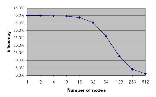
$$\eta_p^{rel} = \frac{S_p^{rel}}{p} = \frac{\frac{T_1}{T_p}}{p}$$
