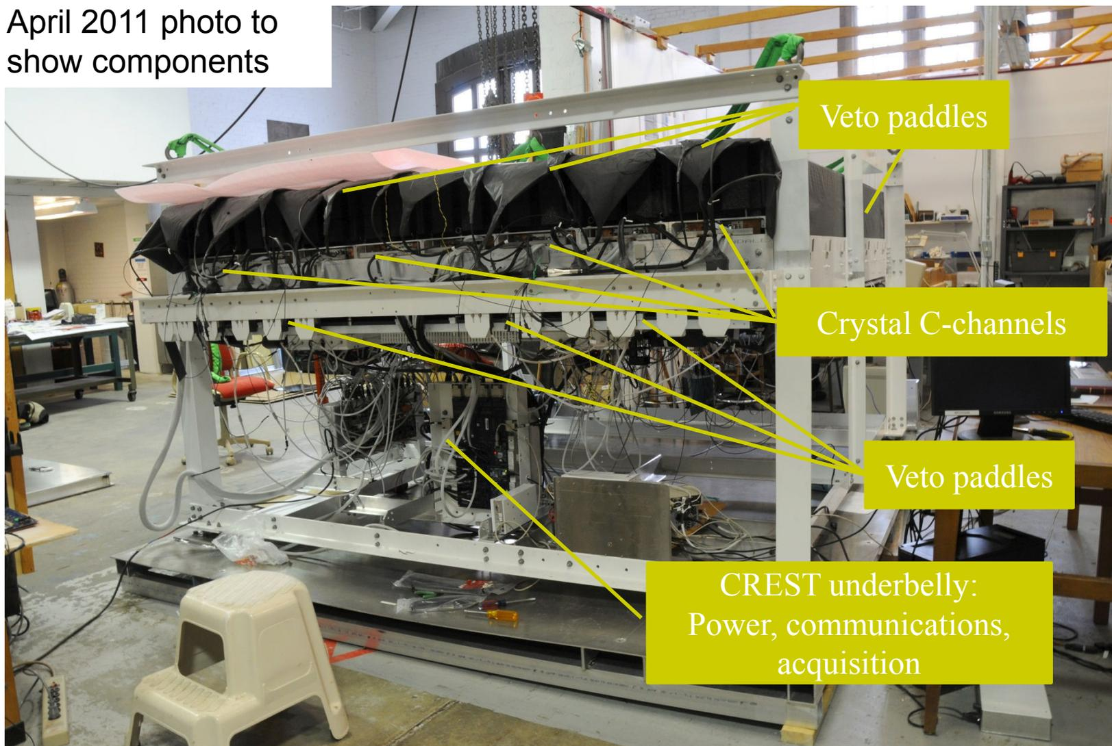
Assembly completed, integration at NASA/CSBF in progress
