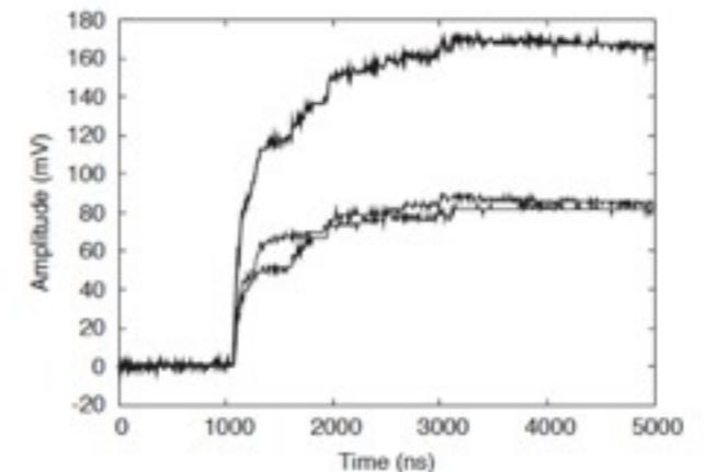
Fig. 4. Event collected in noise measurement experiment mimicking scintillation. As in Fig. 3, the two lower curves show the integrated signals from the individual PMTs. The upper curve shows the sum of these signals.
