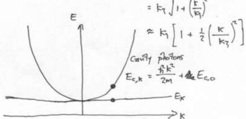
Consider cavity photons & excitons at some given in-plane wavevector
