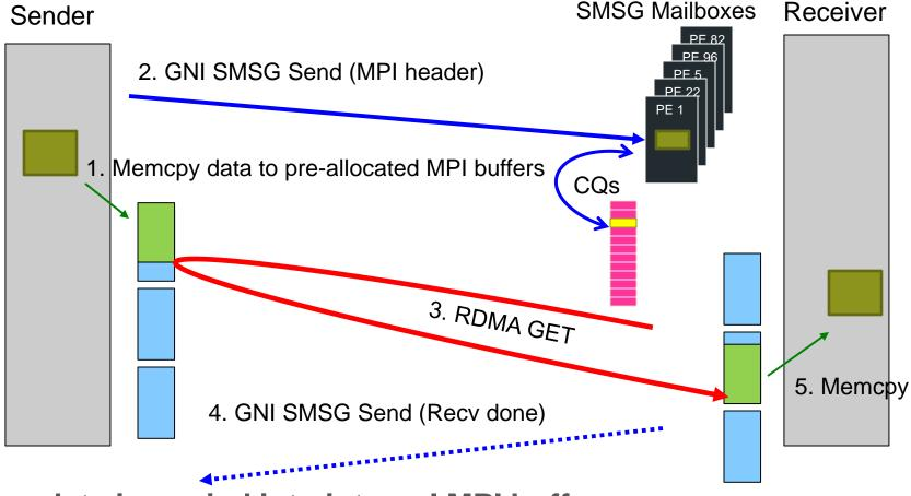
User data is copied into internal MPI buffers on both send and receive side
