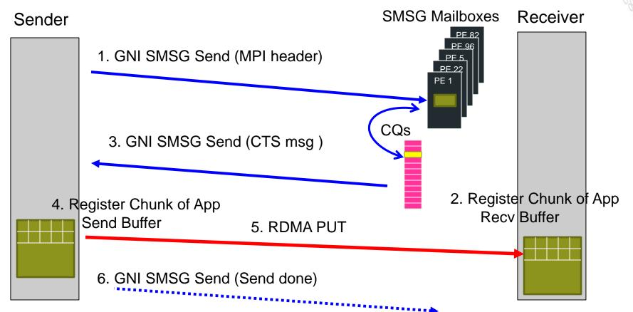
Repeat steps 2-6 until all sender data is transferred Chunksize is MPI\_GNI\_MAX\_NDREG\_SIZE (default of 4MB)
