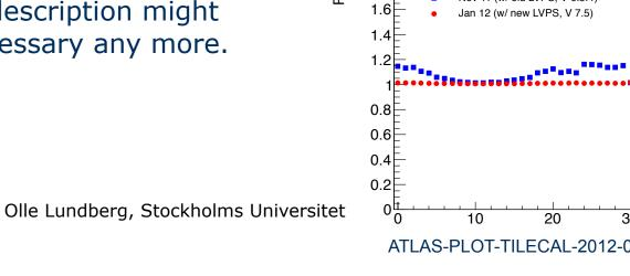
Number of Events BC41. Channel 47 ATLAS Preliminary  $10^{3}$ Tile Calorimeter Nov 2011 w/ old LVPS v 6.5.4 an 2012 w/ new LVPS v 7.5 RMS (old): 29.05 MeV  $10^{2}$ RMS (new): 15.24 MeV 10 -50 50 -150 100 150 ATLAS-PLOT-TILECAL-2012-005 Energy (MeV) RMS/0 Average RMS/ $\sigma$  for all 40 changed LVPS ATLAS Preliminary Tile Calorimeter Nov 11 (w/ old LVPS, V 6.5.4) 30 40 50 **Channel Number** ATLAS-PLOT-TILECAL-2012-002
