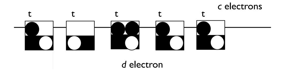
$$H_{KLM} = -t \sum_{rr'} (c_{\sigma r}^{\dagger} c_{\sigma r} + CC) + \sum_{r} (JS_r \cdot S_{d,r} + U_d(n_d - 1)^2)$$
