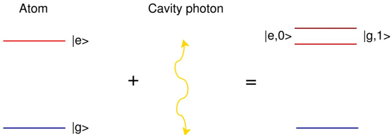
$$\Delta E_{\text{Rabi}}^{\text{JC}} = \sqrt{(\hbar\omega_r)^2 + \delta^2}, \quad \hbar\omega_r = 2g_{\text{EM}}$$
