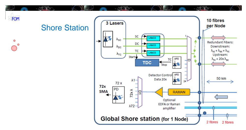
• Slow Control (SC), Detector Control (DC) and Timing Calibration (TC) on 1 separate fiber
