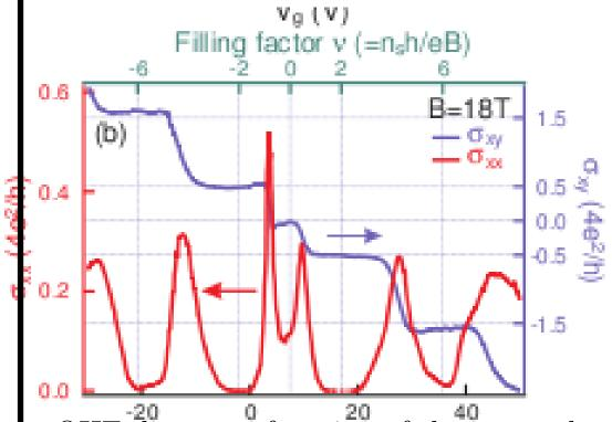
QHE data as a function of the gate voltage  $V_g$ , for B = 18 T at T = 0.25 K
