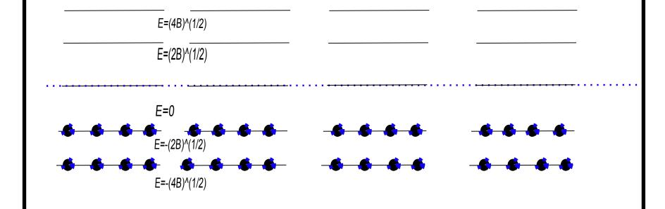
Consider a 4-fold degenerate spectrum of relativistic Landau levels Ground state has negative energy levels filled The zero energy states should be half-filled
