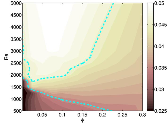
Non-monotonic behavior of the transitional Reynolds number, in line with the experimental observation by Matas et al., sensitive to the chosen threshold as in simulations
