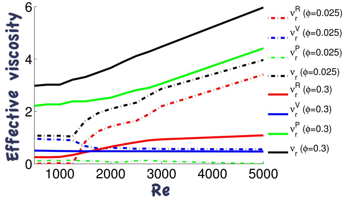
Contributions to the total wall friction due to the viscous, particle and Reynolds stresses for  $\phi=0.025$  and  $\phi=0.3$
