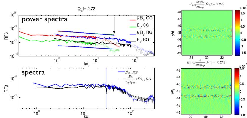
Fig 4: electrostatic (ES) LHDI branch time scales and wavenumbers: Ex  $\delta B_z$  coupling observed, electron current as mediator  $\rightarrow$  break in the  $\delta B_z$  power spectra at lower, non coupled ( $k d_i \sim 30$ ) wavenumbers
