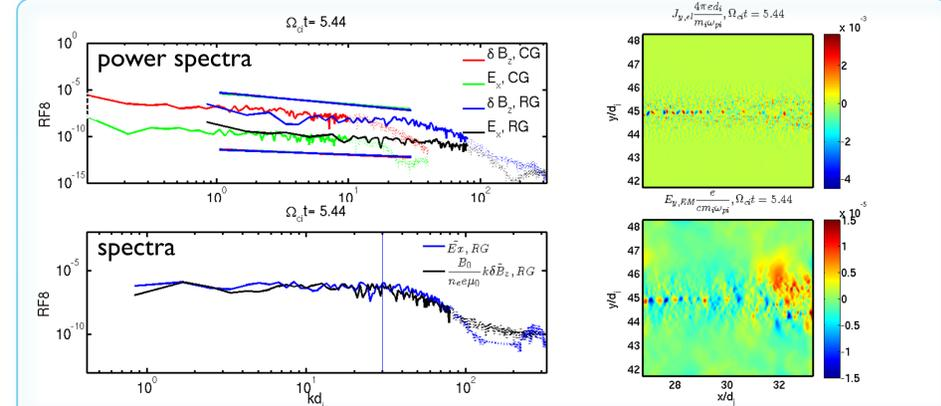
Fig 5: coupling extends to LHDI electromagnetic (EM) wavenumbers with the onset of LHDI EM branch ( $1/\sqrt{(\rho_e \rho_i)} \sim 20/d_i$ ); mediator is still the electron current, but structures are at the centre of the current sheet and of EM origin
