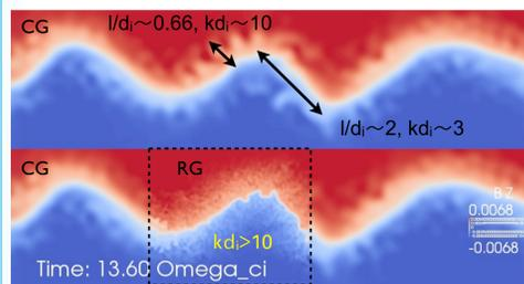
Fig 3: zoom of the out-of-plane field component Bz in a MLMD simulation of LHDI with RF=8; different wavelengths are visible in the Coarse (CG) and Refined (RG) Grid, superimposed in the bottom panel
