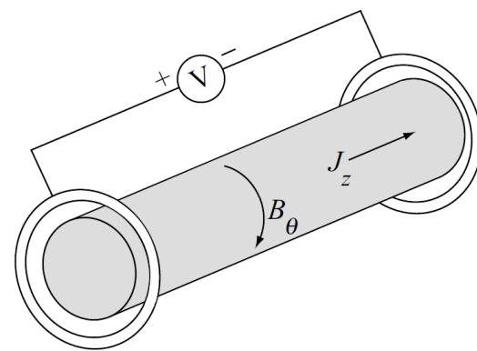
Figure 11.14 Schematic diagram of a Z-pinch.
