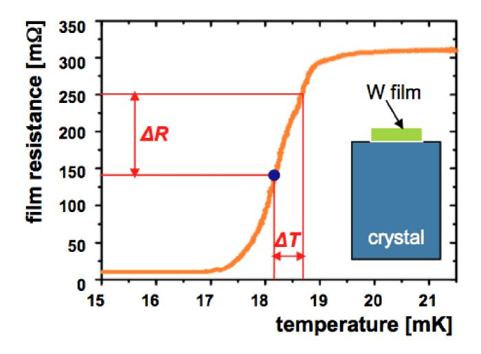
The "superconducting strip" or "transition edge sensor (TES)"
