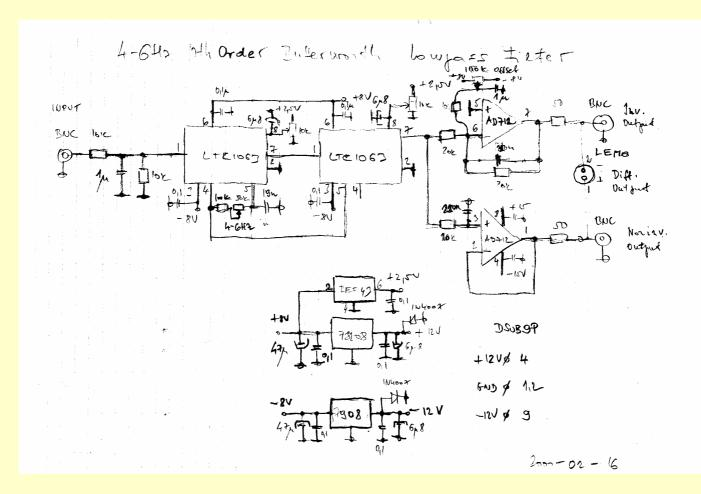
With a potentiometer you can change the upper frequency between 4 and 6 Hz
