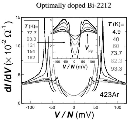
Dynamic conductance of a Bi2212 mesa at different  $T$ . Inset shows detailed curves for high  $T$ . Coexistence of the superconducting peak,  $V_s$ , and the pseudo-gap hump,  $V_{pg}$ , is clearly visible at  $T=77.7$  K.
