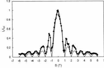
Fig. 2. Magnetic field  $B$  dependencies of critical currents of  $\text{Bi}_2\text{Sr}_2\text{CaCu}_2\text{O}_8$  junctions at  $T = 4.2$  K.  $B$  is parallel to the layers for the junction size of  $1.5 \times 1.5 \mu\text{m}^2$  with a hole of  $\phi = 0.2 \mu\text{m}$ .
