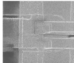
Cutting after deposition of Pt electrodes for true 4-probe measurements
