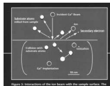
Figure 5: Interactions of the ion beam with the sample surface. The unique control offered by beam currents and spot sizes allow use of the FIB for both nano engineering as well as for high resolution imaging using secondary electrons as well as ions.
