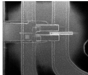
Cutting and deposition of extra contact electrodes (Pt) by FIB
