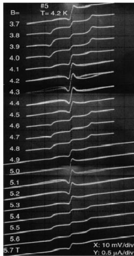
Fig. 7. A set of the  $I$ - $V$  characteristics of a short Bi-2212 stack #5 with variation of parallel magnetic field  $B_{\parallel}$  within 3.7-7.5 T,  $T = 4.2$  K. Note a Fiske step at  $V \approx 15$  mV.
