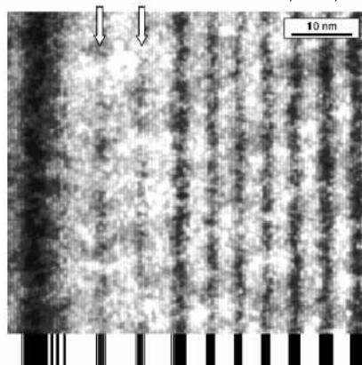
FIG. 1.  $60 \times 60 \text{ nm}^2$  filled states STM image of the graded structure with layer sequence indicated at the bottom of the image,  $V_{\text{sample}} = -1.6 \text{ V}$ . The black layers are the InAlAs barriers and the white layers are the InGaAs wells. P.Offermans et al., Appl.Phys.Lett. 83 (2003) 4131
