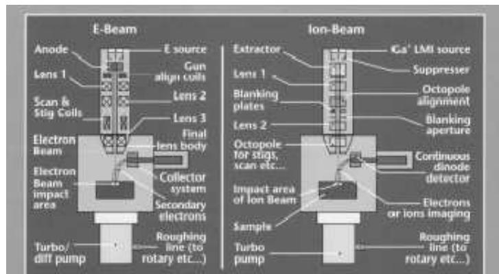
Figure 6: Schematic presentation of SEM and FIB and the many similarities of the instruments.
