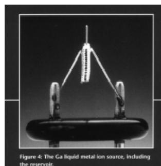
Figure 4: The Ga liquid metal ion source, including the reservoir.
