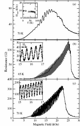
FIG. 2. Flow resistance of Josephson vortices as a function of magnetic field of samples A (a), B (b), and C (c) with an applied current of 1, 1, and  $10 \mu\text{A}$ , respectively. The inset of (a) shows the temperature dependence of  $H_{\text{max}}$  for sample B. The enlarged figures of the flow-resistance oscillations of samples B and C are shown in the insets of (b) and (c), respectively.
