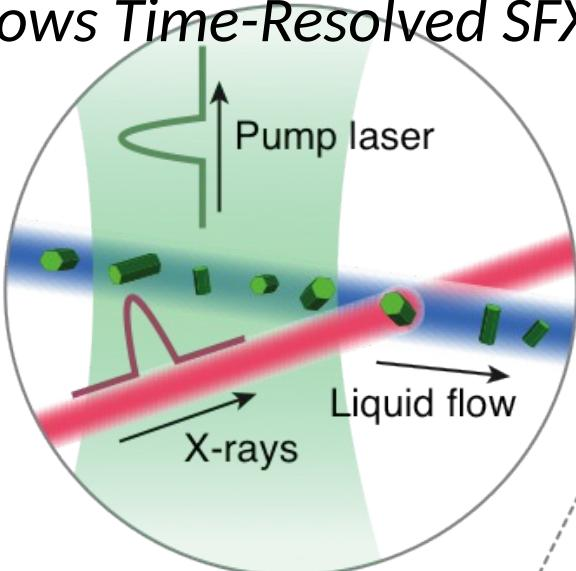
The 10 fs XFEL pulses should allow us to improve on the ~ 100 ps time resolution of SR (at RT, without damage).
