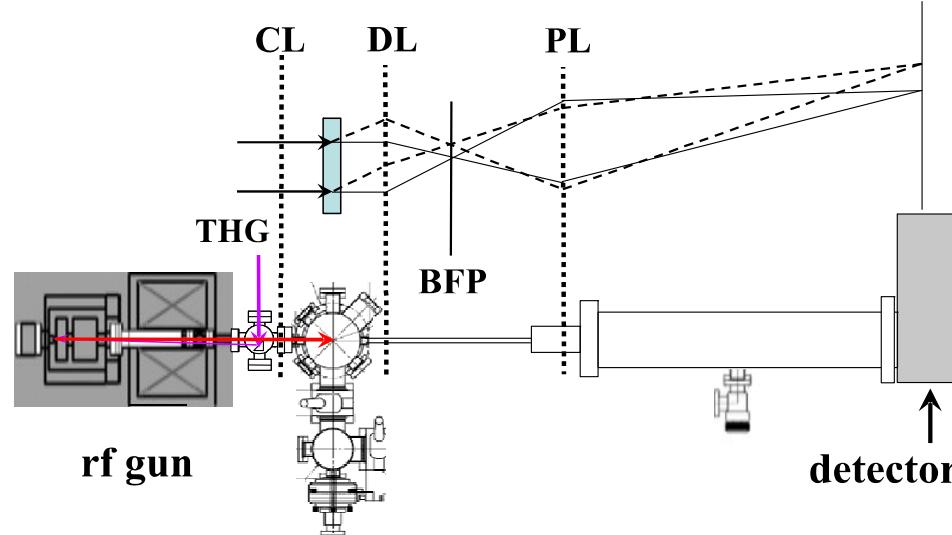
**Electron Diffraction Camera.** 3 MeV,  $1.06\text{E}6 \text{ e}^-/\text{pulse}$ , 100 fs,  $500 \mu$  beam
