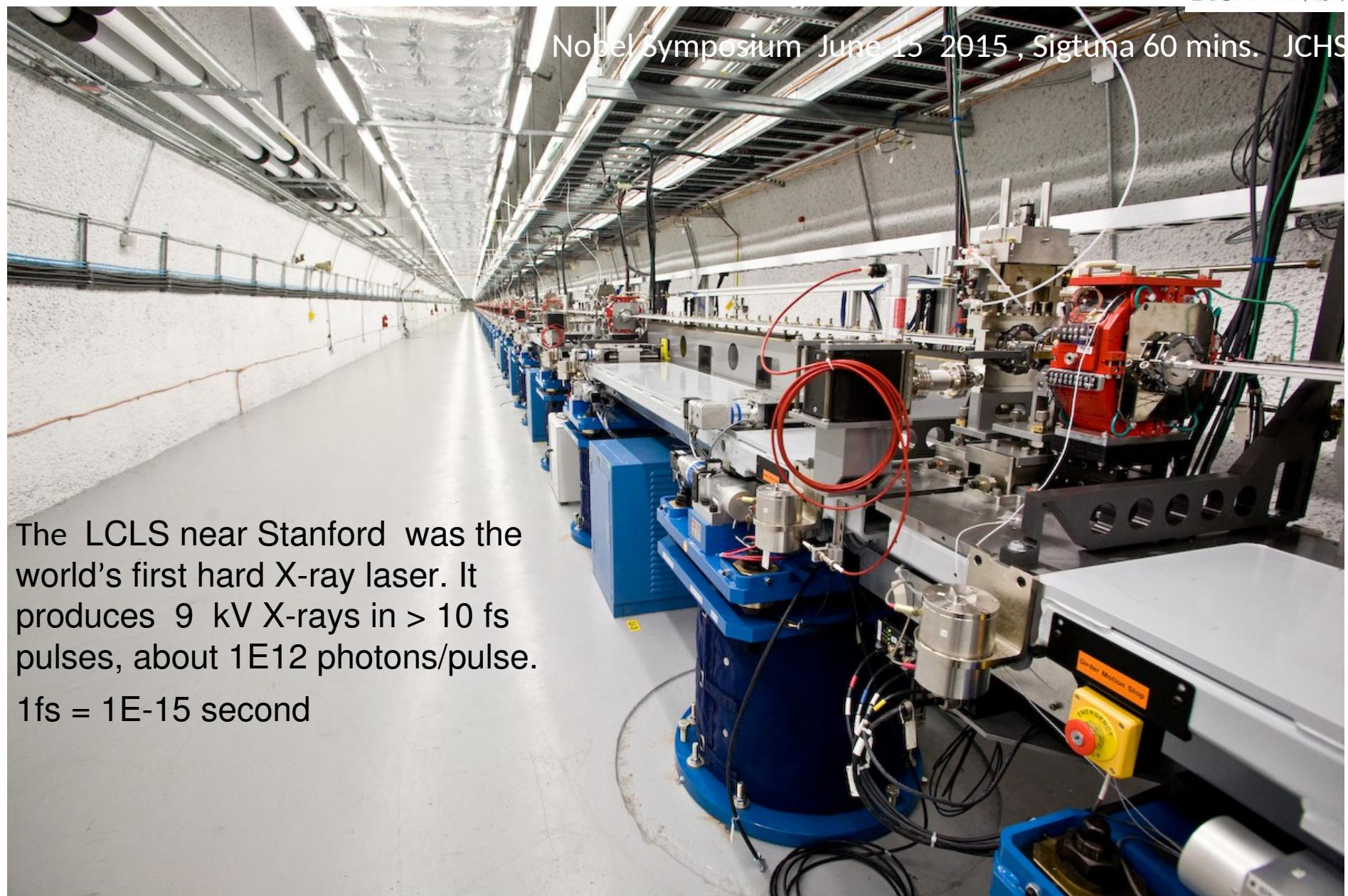
The LCLS near Stanford was the world's first hard X-ray laser. It produces 9 kV X-rays in  $> 10$  fs pulses, about  $1E12$  photons/pulse.
