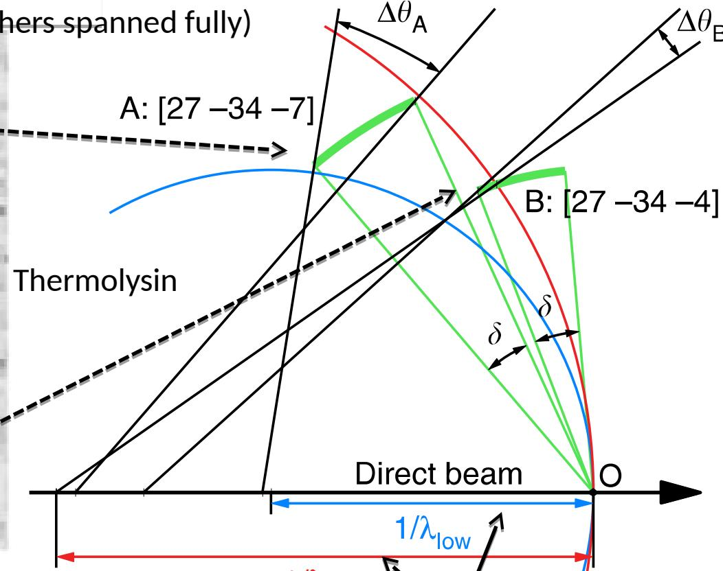
Each tilted mosaic block acts as a monochromator for a different component wavelength in the beam..
