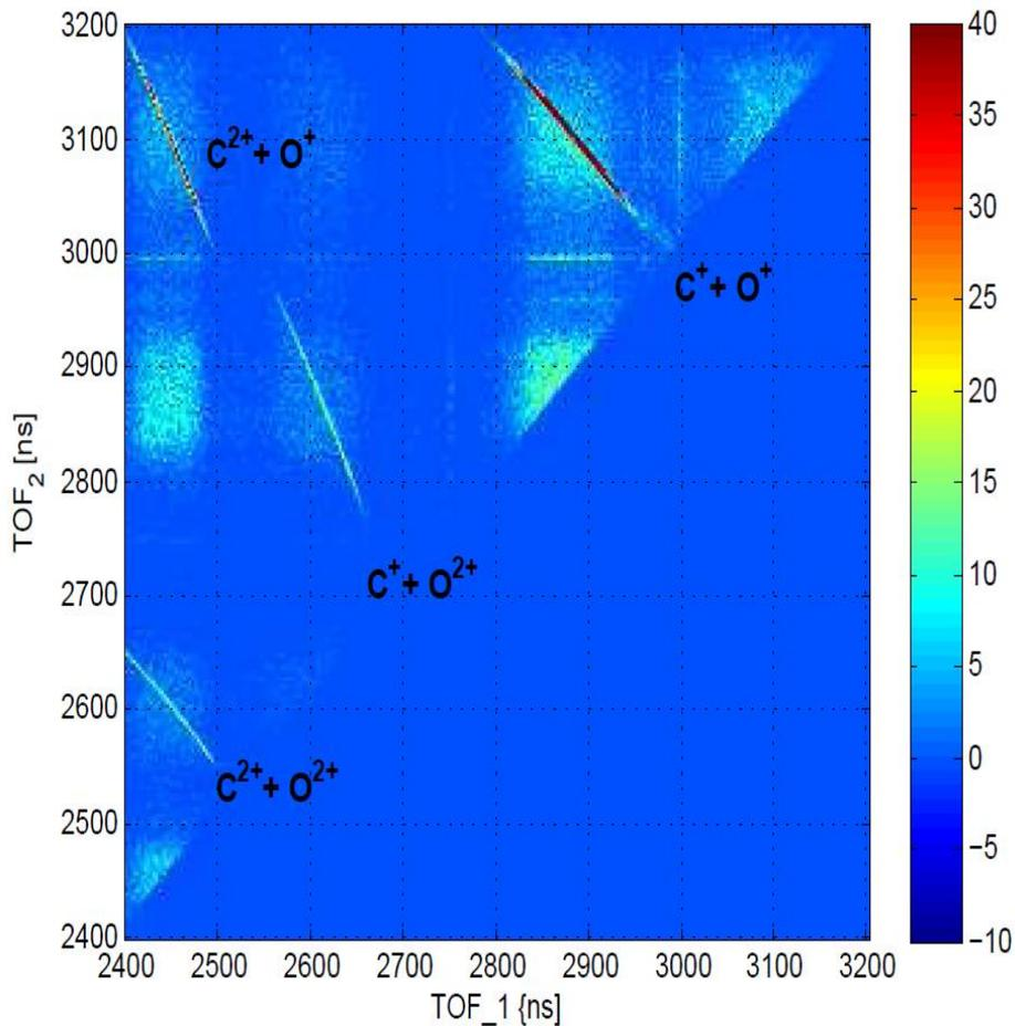
*Ion-Ion Coincidence Events recorded during ionization of CO with 430 eV X-rays with 5fs pulse duration.*
