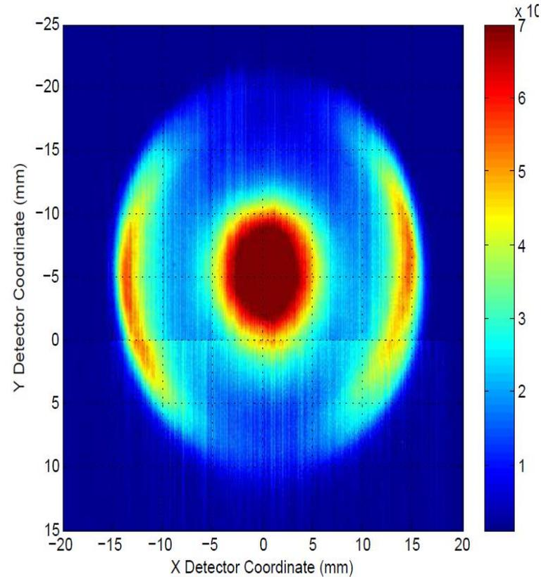
*Electron spectra recorded for ionization of Ne. Outer ring: Ne 1s photoelectron dipole angular distribution.*
