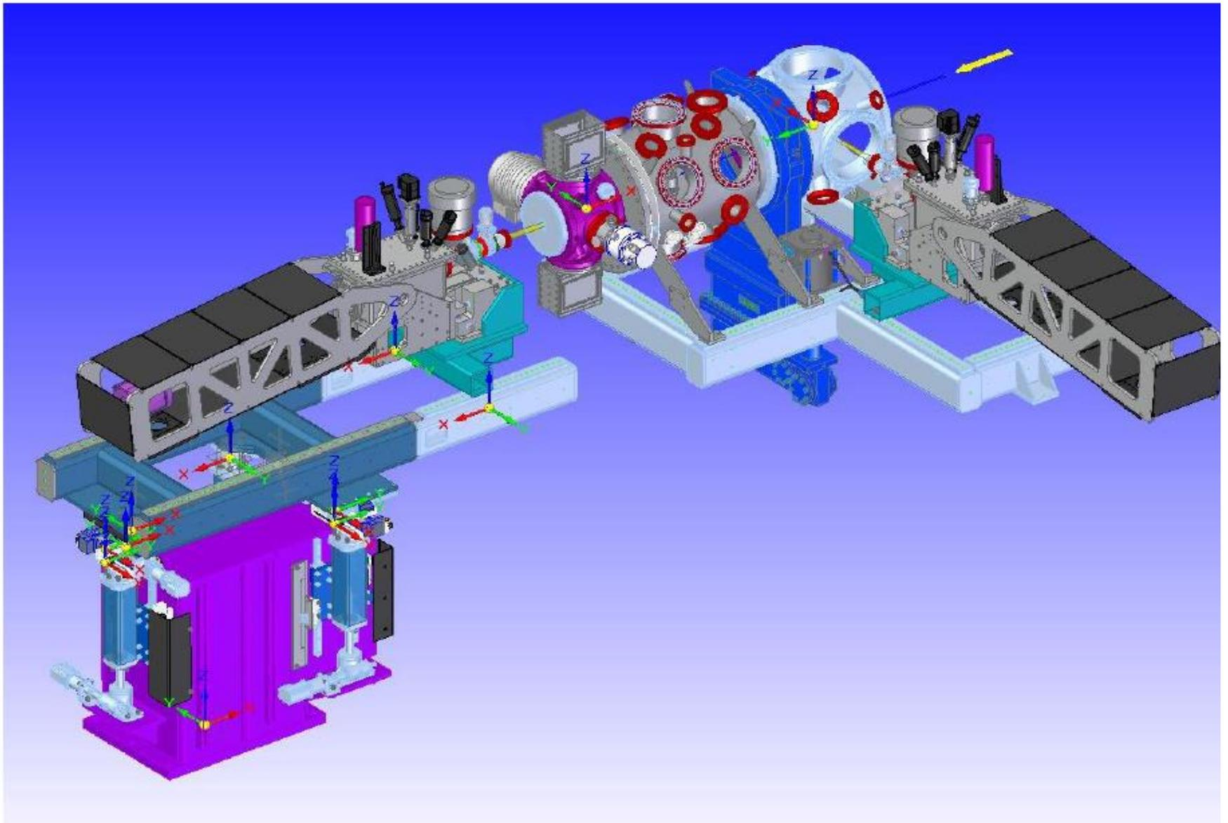
Figure 1: CAD model of the spectrometer installed on the AMO LAMP instrument. Two configurations, forward and  $90^\circ$  horizontal are shown.
