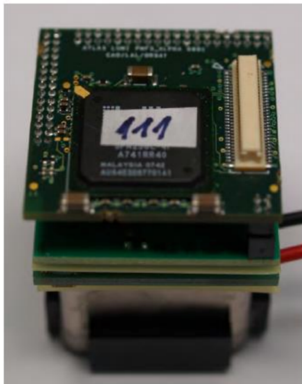
Figure 14.6. LEFT : MAPMT with full PMF mounted: MAPMT + isolator + spacer + voltage divider + spacer + isolator + passive board + active board. RIGHT : The layout of the MAROC 2. The figure is figure 3 in [58]. The red numbers are added to the figure.
