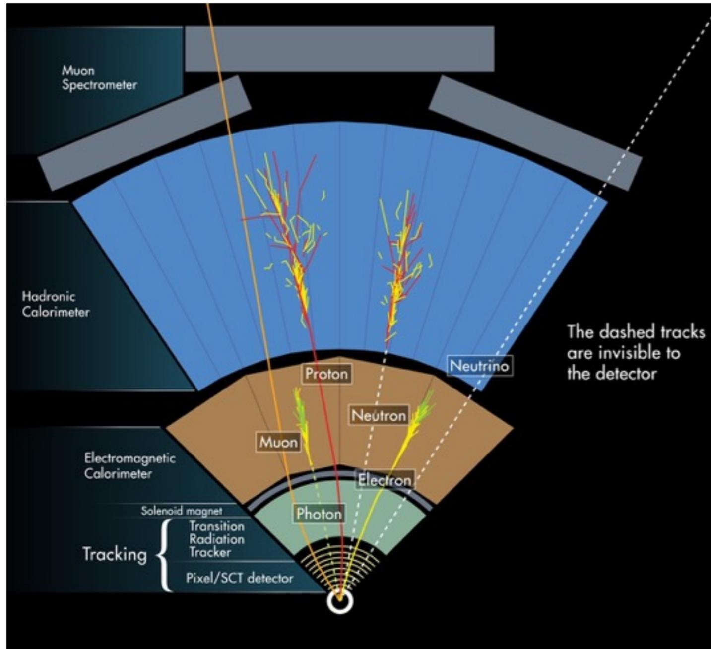
A cross sectional diagram of the ATLAS detector with various particle trajectories (photo from [atlasexperiment.org/photos](http://atlasexperiment.org/photos))
