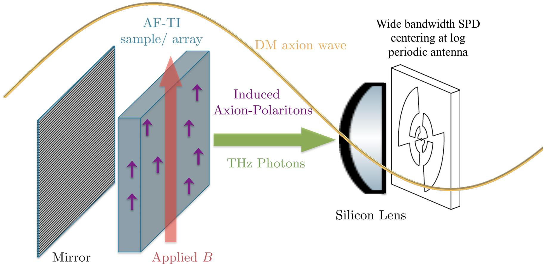
Dark count rate 0.001 Hz demonstrated at 0.05 K with Quantum Dot Detector. Need wide bandwidth version.
