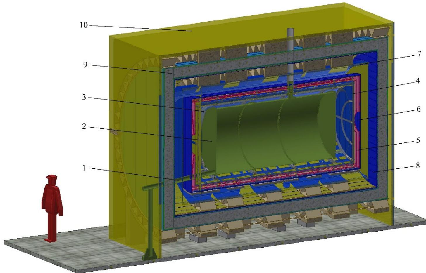
1 – neutron guide, 2 - UCN trap, 3 - vacuum chamber, 4 – trek detector (inner part), 5 - magnetic shield, 6 - hodoscope (internal part), 7 - trek detector (middle part), 8 - hodoscope (external part), 9 - calorimeter, 10 – active shielding
