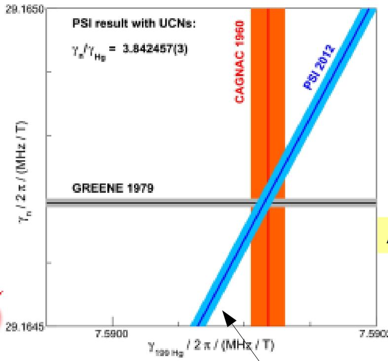
Super precise measurement of magnetic moment of neutron relative to proton by Geoff Greene
