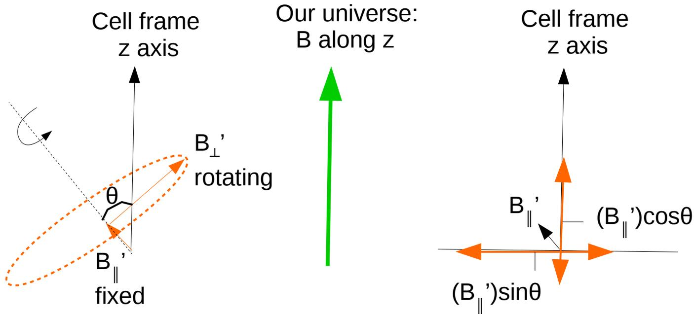
The cell sweeps out a trajectory, where  $B_{\parallel}'$  is constant, and  $B_{\perp}'$  rotates at frequency  $\Omega$
