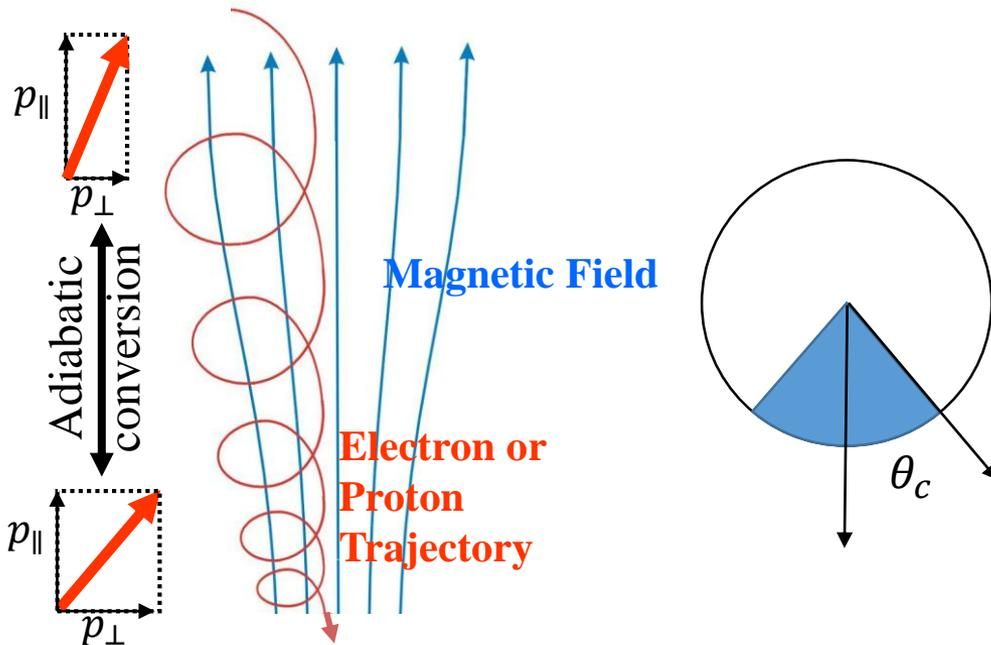
If  $B_{filter} > B_{decay}$ , detector behind filter detects only particles with angle to field  $\theta$
