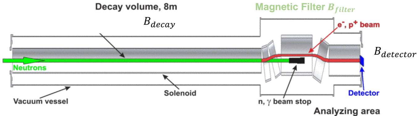
**Active volume** in a 8 m long neutron-guide,  $B_{decay} \leq 1.5$  T:
