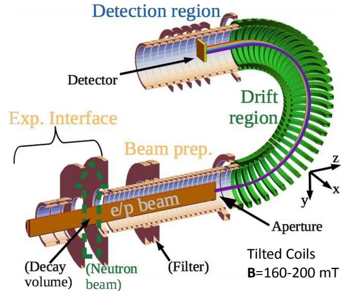
R×B Magnet is planned to be available at the end of 2020. Nomos is planned to be used to determine  $a$  and  $b$  to 0.1% level.
