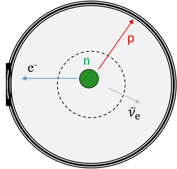
Surface: position-sensitive electron+proton detectors (E/P detectors),  $4\pi$  coverage
