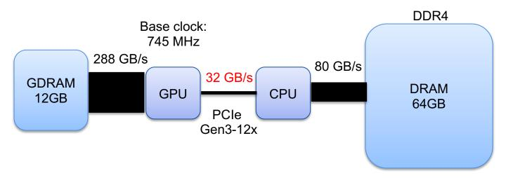
NVIDIA TESLA K40 = the most common GPU on supercomputers in Nov. 2016 Top500 list
