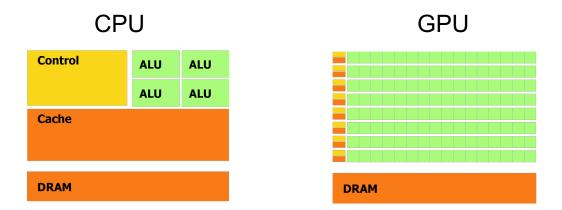
CPU has tens of massive cores, CPU excels at <u>irregular control-intensive</u> work
