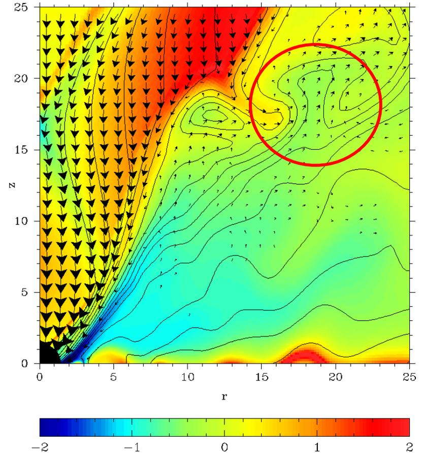
The disk accretion makes easier the explosion conditions. The MF lines shape reduce local accretion rate.
