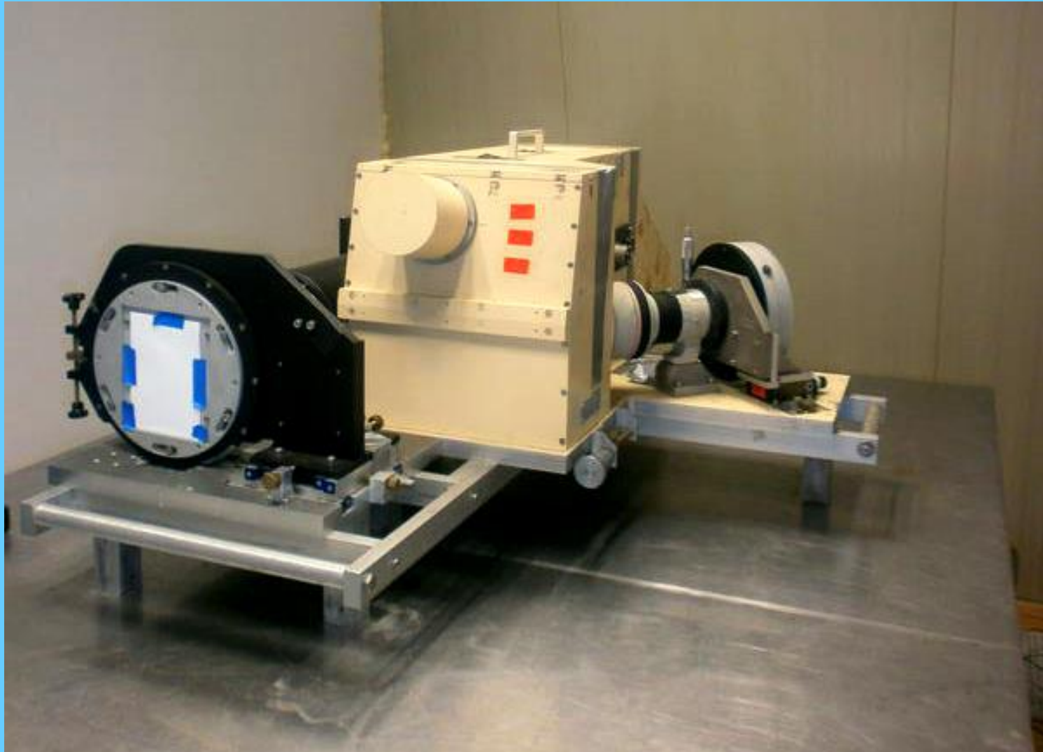
HEROS: fiber-fed Spektrograph (L.Stw. Heidelberg), air-conditioned and stable table, R=21.000 in red and blue channel, to \sim 10 mag
