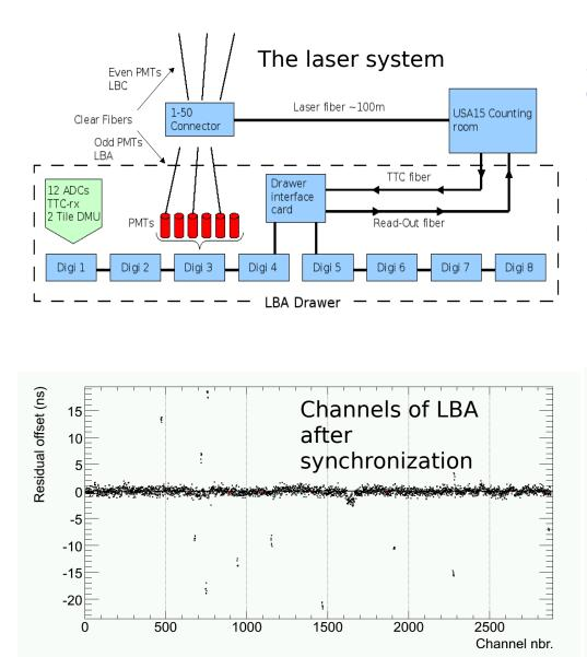
B. Nordkvist, C. Clement For an optimal energy and time reconstruction TileCal readout must be synchronized to a precision of < 2 ns w.r.t clock signal
