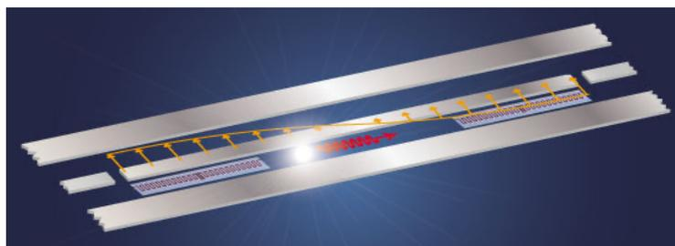
SAW coupled atoms are larger than the wavelength of SAWs
