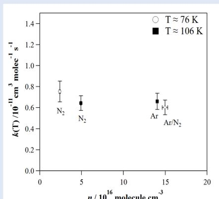
Figure 5b. Pressure dependence of  $k(T)$  at 76 and 106 K.
