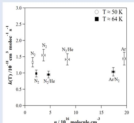
Figure 5a. Pressure dependence of  $k(T)$  at 50 and 64 K.
