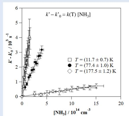
Figure 3.  $k' - k'_0$  versus  $[NH_3]$  in the jet for 3 different temperatures.
