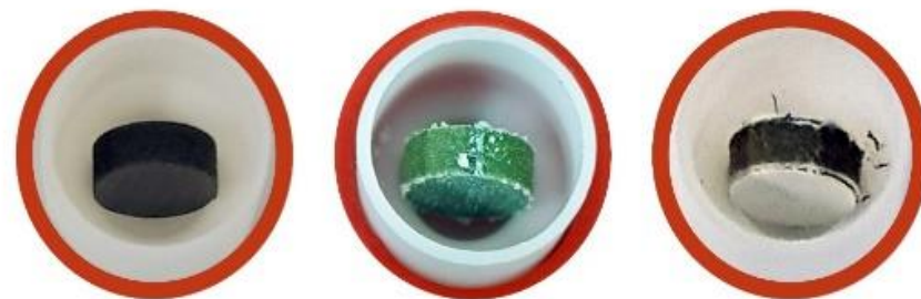
Ta2.5W degradation at different temperatures under oxidizing atmosphere
