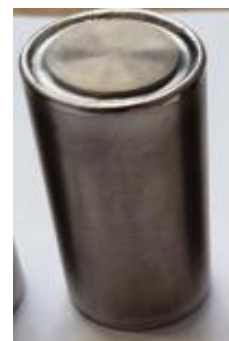
Successfully bonded Nb-alloy cladded block. UT imaging
