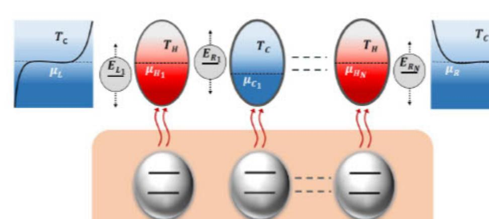
Thermal control across a chain of electronic nanocavities
