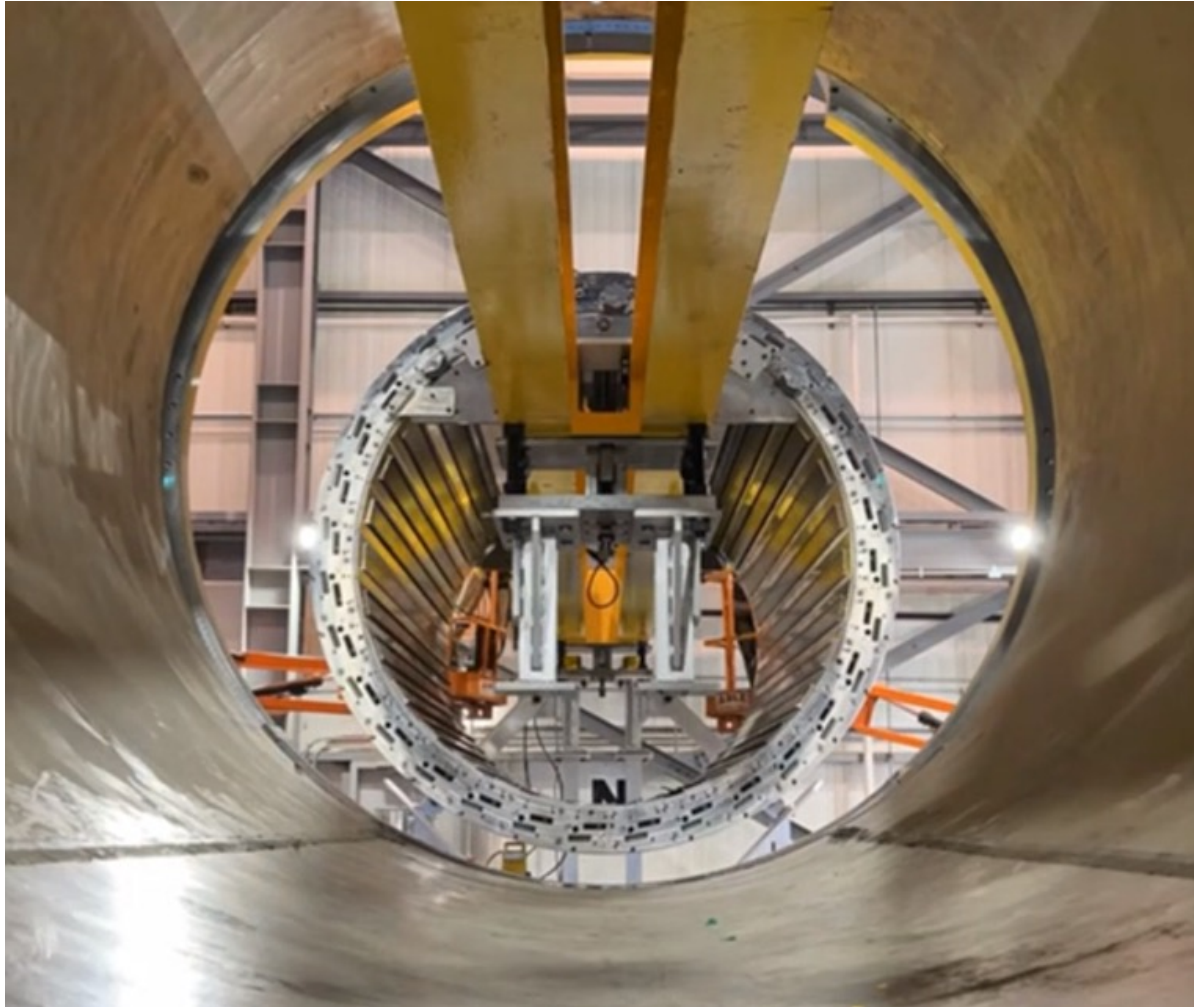
Left: Inner hadronic calorimeter installation, June 2022
