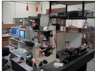
Figure 2.9: This photo was taken in June 2005, after the system was significantly modified. The components in the photo are: (1) Nikon Diaphot 300 inverted microscope, (2) Microscope objectives, (3) Microscope stage, (4) Coherent Compass 4000M Laser, (5) BEOC Laser Stabiliser, (6) MTI IFG CCD Camera, (7) Physik Instrumente Piezo Translator, (8) replacement control computer with custom written
