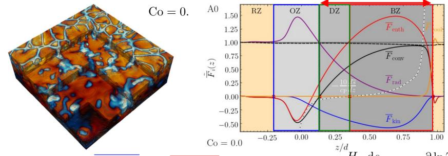
$$\overline{F}_{\text{conv}} = \overline{F}_{\text{kin}} + \overline{F}_{\text{enth}} = \frac{1}{2} \rho \mathbf{u}^2 u_z + c_{\text{P}} \overline{(\rho u_z)' T'}, \quad \Delta \nabla = \nabla - \nabla_{\text{ad}} = -\frac{I}{c_{\text{P}}} \frac{\mathrm{d}s}{\mathrm{d}z}, \quad \nabla = \frac{\partial \ln T}{\partial \ln p}.$$
