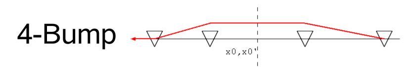
Use four steerers to adjust angle and position at a center point and then flatten orbit downstream of the last steerer.
